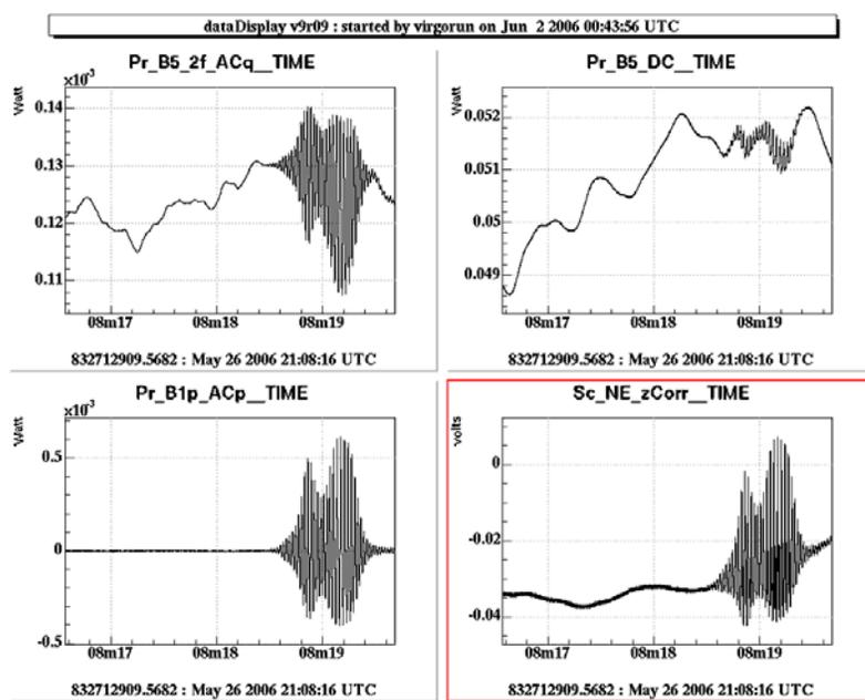
Typical interferometer Oscillations in the region 30-50 Hz in the sidebands power (upper left), carrier power (upper right), differential arm error signal (lower left) and differential arm control signal (lower right)
