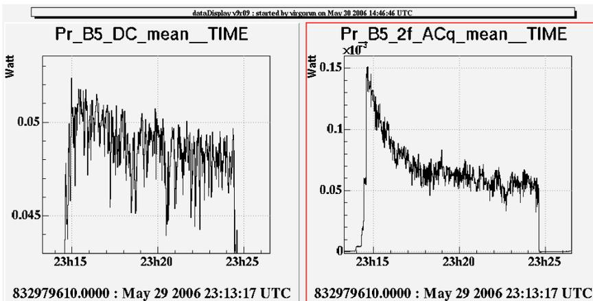
Carrier power (left) and sidebands power (right) over ~15 minutes of lock.
