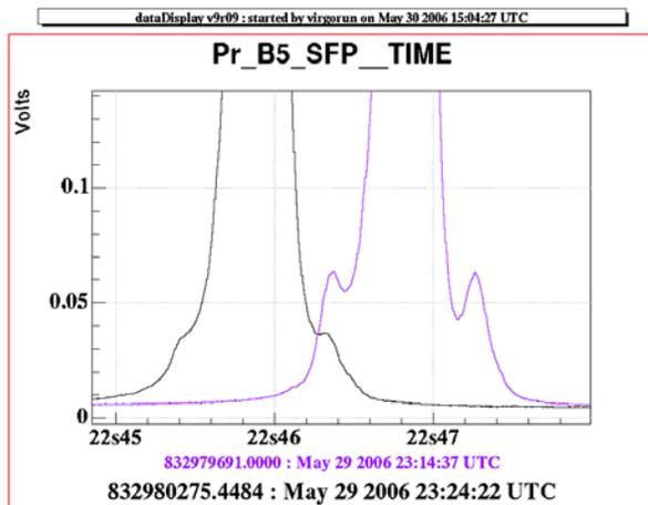
Another (more direct) measurement of the sidebands decrease: optical spectrum taken with a scanning Fabry-Perot on the pick-off beam of the interferometer (B5), at the beginning of the lock (purple) and at the end (black). The big peak is the carrier, and the small lateral peaks are the sidebands.
