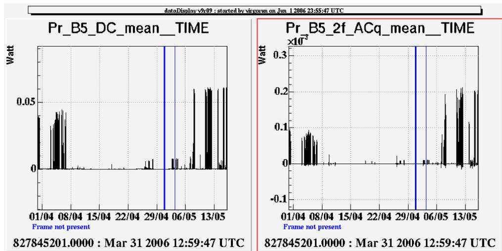
Trend of data before and after the mirror centering: the left plot is the carrier stored power and the right plot is the sidebands one. After the centering (at the beginning of may), the carrier power increased by a factor 1.5 and the sidebands power by a factor 2.
