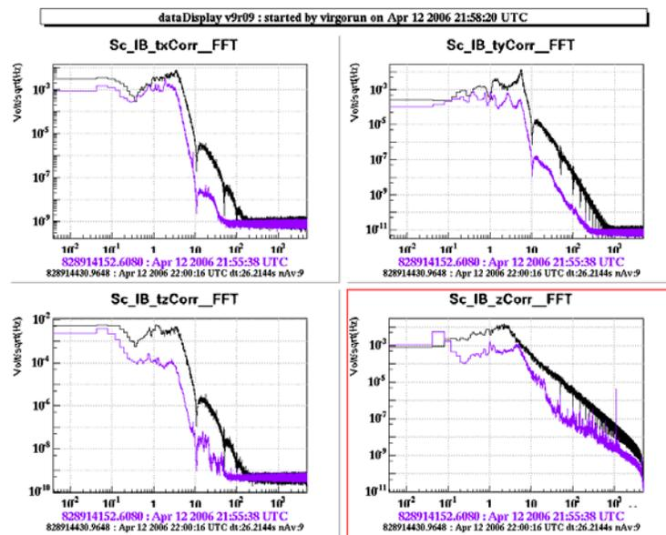
Correction signals for the four degrees of freedom concerned by the new IB autoalignment system (first attempt of implementation). Black: IB under local control; blue: IB under autoalignment.
