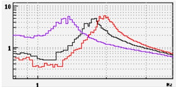
*Zoom on the transfer function of the  $\theta_y$  (yaw) degree of freedom of the mode cleaner mirror. The measurement was made with zero (purple), 70% (black), and 100% power in the mode cleaner cavity; the resonance frequency shifts correspondingly.*
