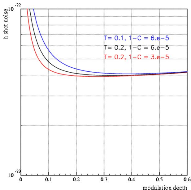
Figure 2: Projection of B1 shot noise on Virgo sensitivity as a function of the modulation index for a recycling gain  $R=31$  as measured on the data and 3 plausible combinations of sidebands transmission ( $T$ ) and contrast defect ( $1-C$ ). The modulation effect is taken into account. These curves have to be multiplied by the cavity transfer function (cut off at 500 Hz) in order to get the shot noise limited sensitivity for a given frequency.
