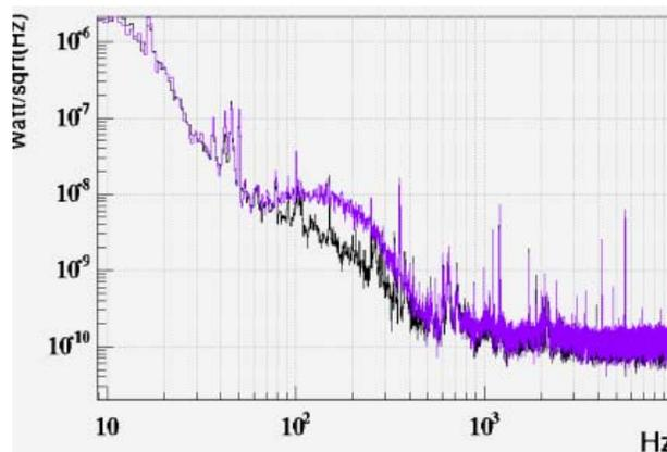
*Fig.4.3 - Evidence of diffused light effect on dark fringe spectrum (black curve measurement after installation of a beam dump)*
