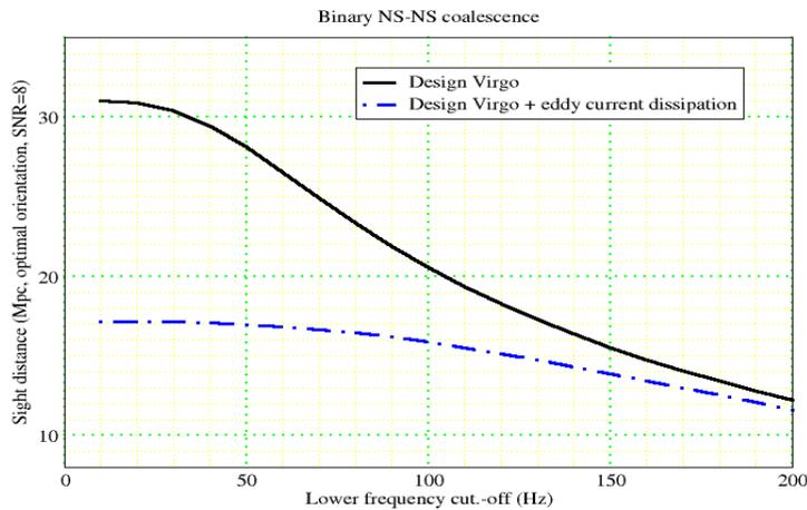
Fig 4.1 Horizon for NS-NS inspirals (in Mpc) vs lower frequency cut-off (in Hz) for the 2 configurations of Virgo design and Virgo design + eddy current dissipation
