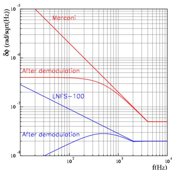
Figure 1: Signal generator phase noise for both Marconi (red) and LNFS-100 (blue) according to their respective specifications. In the two cases the upper curve gives the intrinsic generator phase noise (as given by the constructor) and the lower curve gives its projection on the dark fringe, i.e. after demodulation.
