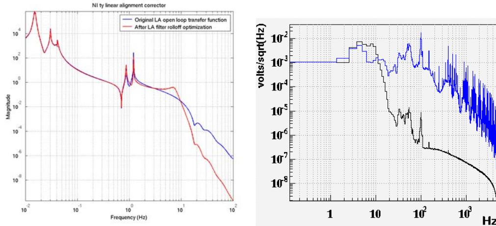
**Figure:** A comparison of the open loop transfer function of the horizontal angular degree of freedom of the North input mirror (left), and of the total control noise going to the coil actuators (right), before (blue), and after the optimization. The improvement is two orders of magnitude at 30 Hz, and four at 100 Hz.
