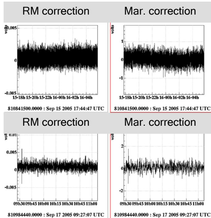
Figure 4.3: the upper figure shows the maximum value of the correction signal on the reference mass and the marionette respectively on a long stretch of data (12 hrs) in science mode during C7. The typical value on the RM is 3 mV (to be compared with a saturation level of 16 mV!). Notice that during C7 the WE mirror was not controlled. The marionette correction is below 1 V, showing that it is possible to increase the amount of correction reallocated upon the marionette.
