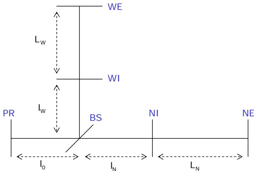
Fig.3.1 – The interferometer longitudinal degrees of freedom.
