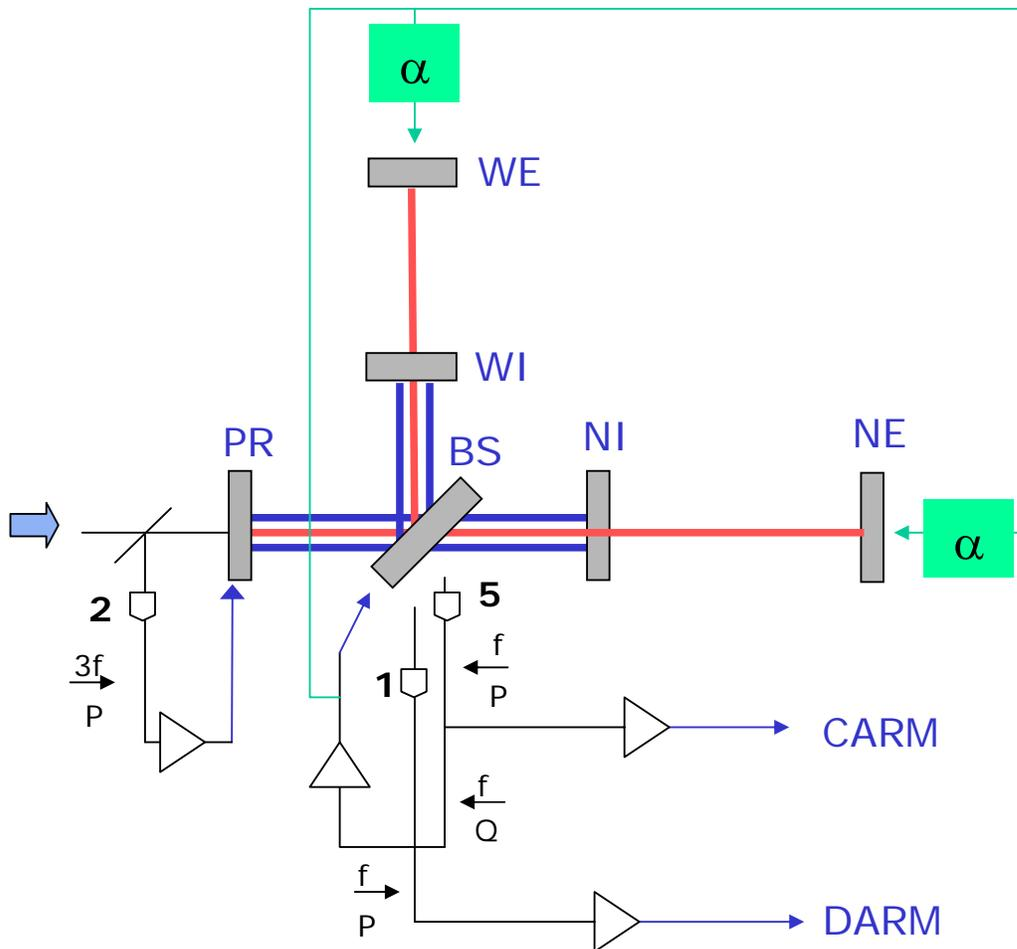
Fig.4.6 – Scheme of the BS noise subtraction
