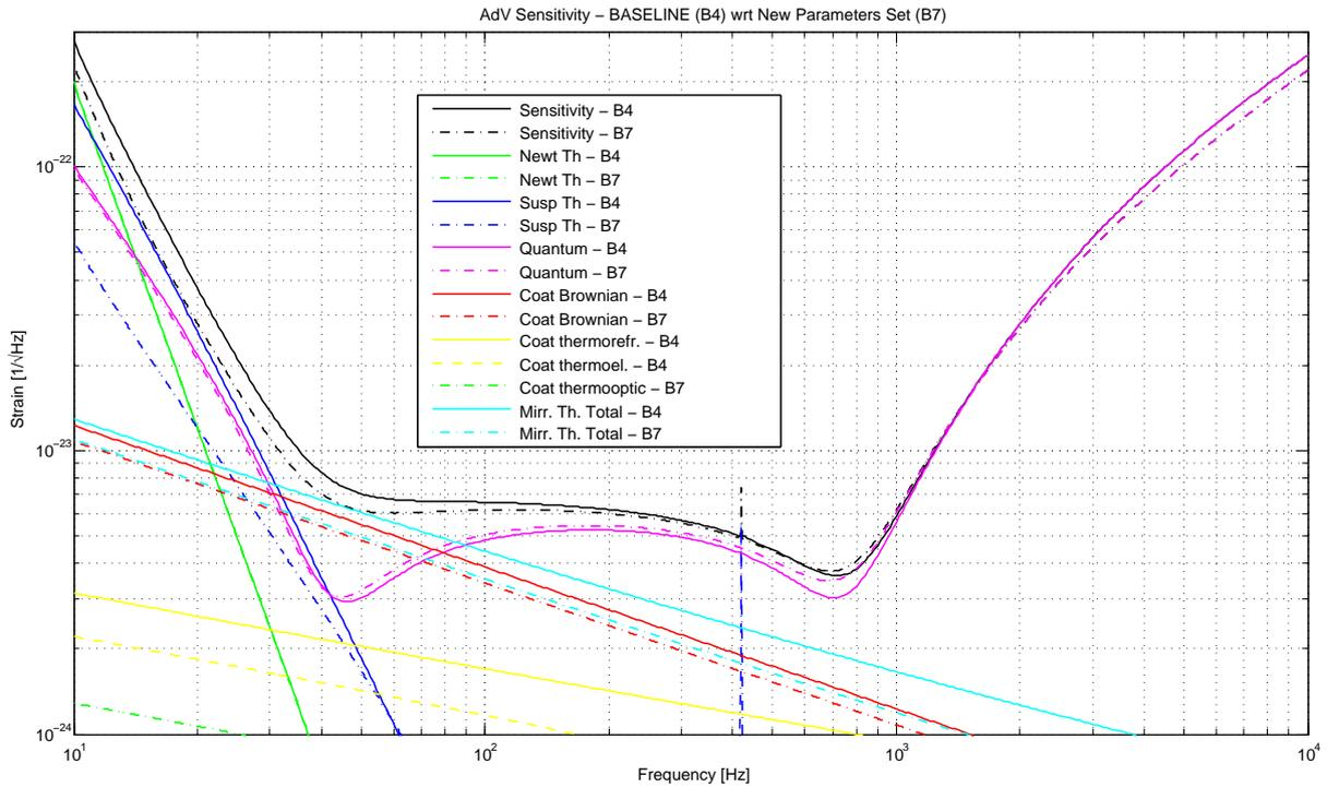
Figure 2: AdV baseline sensitivity from [1] (traces labeled B4, baseline scenario) and the new reference sensitivity, calculated with GWINC and using the parameter set described in Section 5 of this document (traces labeled B7, new reference scenario). The corresponding input files are IF0Model\_conceptual\_design.m for B4 and adv\_27062008.m for GWINC.
