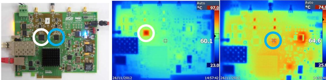
*Figure 7 Left: regular image of the test board. Centre: thermal image with the ADS5474 turned on. Right ISLA214 turned on. The white and blue circles indicate the positions of the ADS5474 and ISLA214.*
