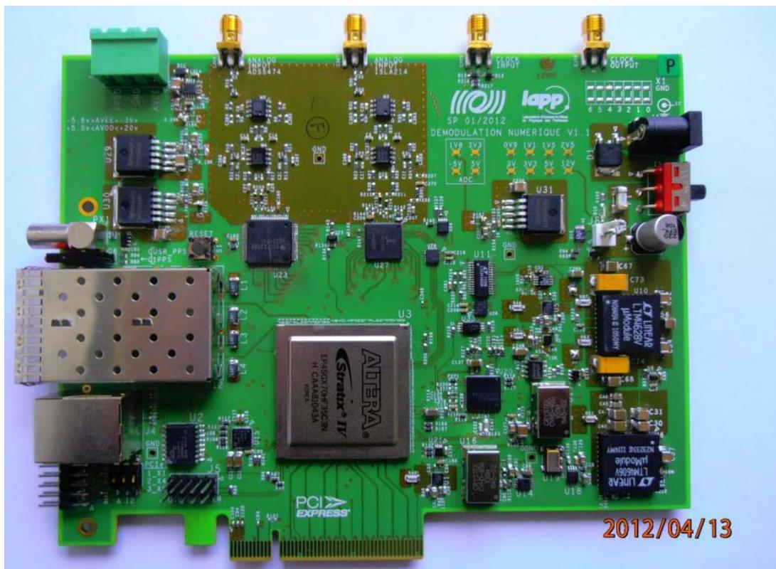
Figure 1 Image of the demodulation test board
