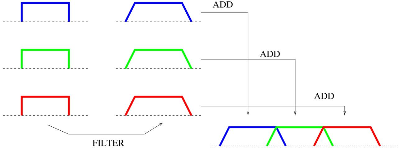
Figure 1: The simulation algorithm. A dashed line represent  $N$  buffers. A dotted line represent  $N$  output streams.
