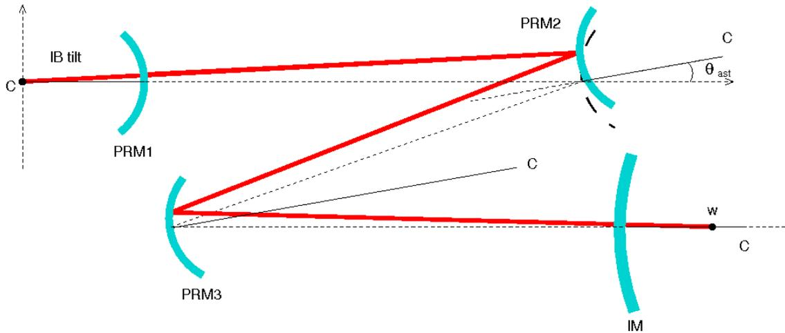
Fig 3.3: a sketch of the geometrical computation of the optical axis for the power recycling cavity
