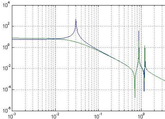
*Fig 3.2: Mechanical transfer function of the Super Attenuator with a radiation anti-spring as present in Virgo+. The 30 mHz resonance frequency  $T_y$  mode is brought to instability but the corresponding poles have frequency sufficiently low and the overall system is not affected.*
