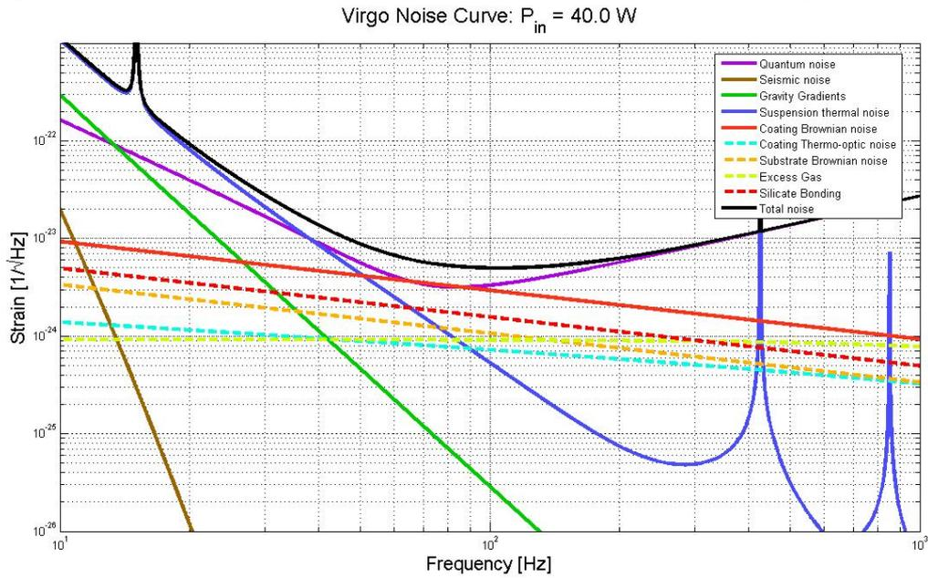
Fig. 4.2 Sensitivity of a bi-concave 40 Watt input power 40 recycling gain without signal recycling. The horizon is 108 Mpc.
