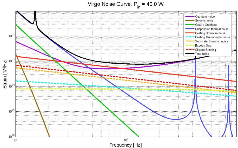
*Fig 4.1: fundamental noises in an interferometer without signal recycling, with 40 Kg masses, cryotrap, higher power and recycling gain. Coating layer optimized, estimated 80% (in power spectral density) with respect to non-optimized. The NSNS horizon is 80 Mpc.*
