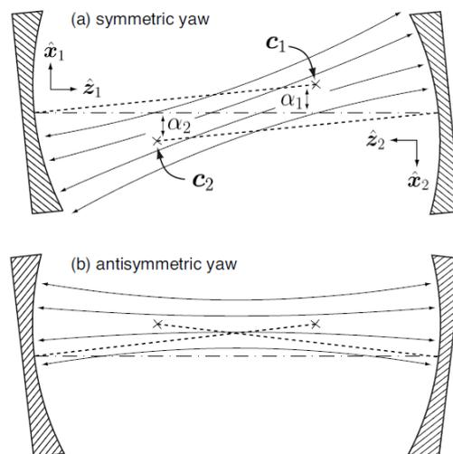
*Fig 3.1: Position of the cavity axis due to rotations of the mirrors. In the picture it is seen that the symmetric yaw exhibits a restoring momentum while the antisymmetric yaw corresponds to an unstable mode.*
