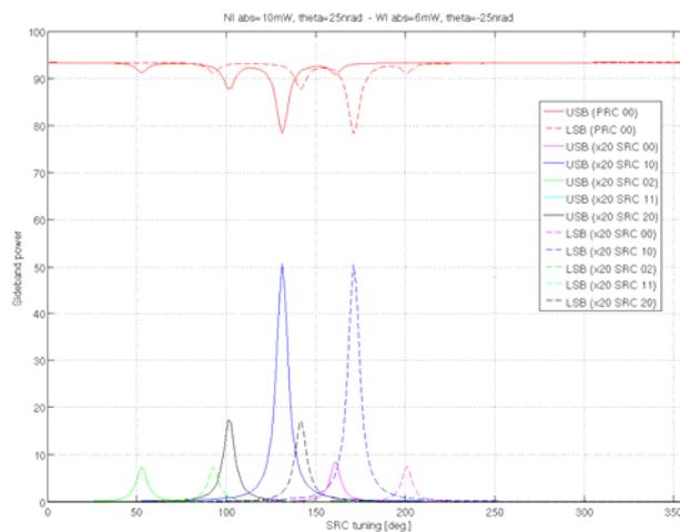
**Figure 2 Effect of differential lensing and mis-alignment on the power recycling gain of 6MHz sidebands, as a function of SRC tuning.**
