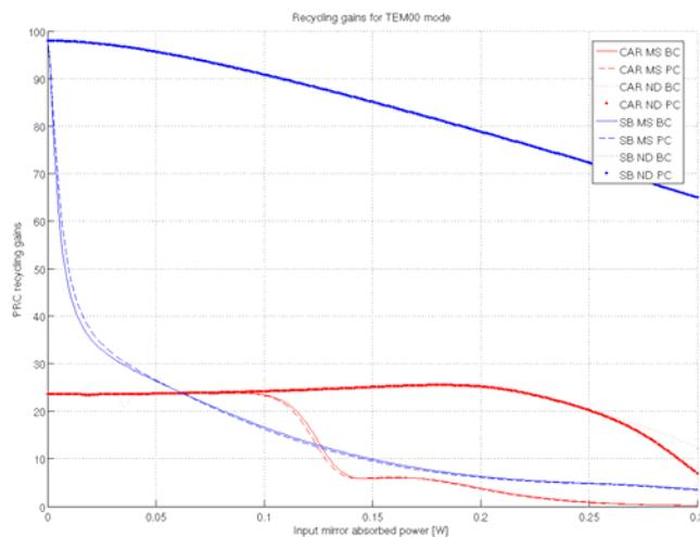
**Figure 1: Comparison of carrier and sideband recycling gains as a function of common mode thermal effects.**
