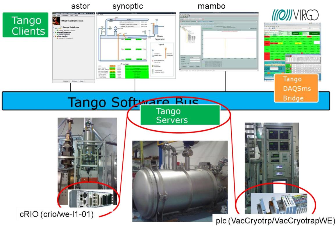
Figure 2 Tango Clients and Servers for the cryotrap control at west-end
