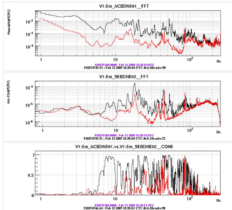
**Figure 2.** Noise reduction consequent to the switch-off of the WE hall air conditioning (black to red). TOP = acoustic noise, MIDDLE = seismic noise at WE bench top, BOTTOM=coherence of the two.
