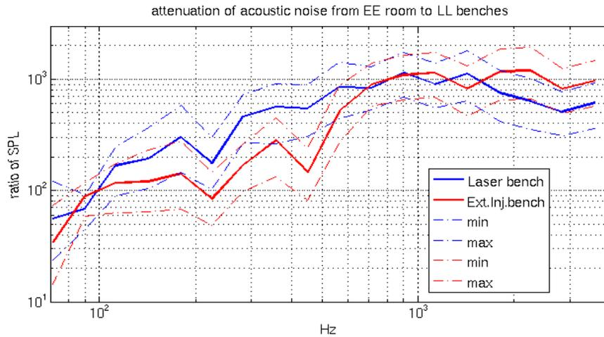
**Figure 7.** Acoustic noise attenuation between the EE-room and the laser benches (inside acoustic enclosure).
