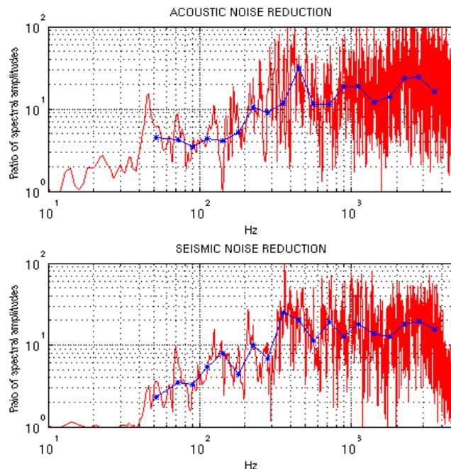
**Figure 6.** Acoustic and seismic noise attenuation of external detection bench provided by the acoustic shield of detection room.
