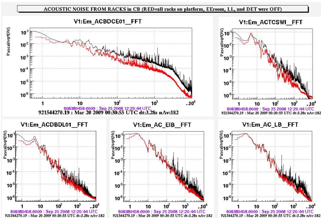
**Figure 8.** Acoustic noise produced by racks in the central experimental hall. Red curves correspond to all racks in LL, DET, and Central hall platform switched off. Some residual noise from DAQ room racks was present.
