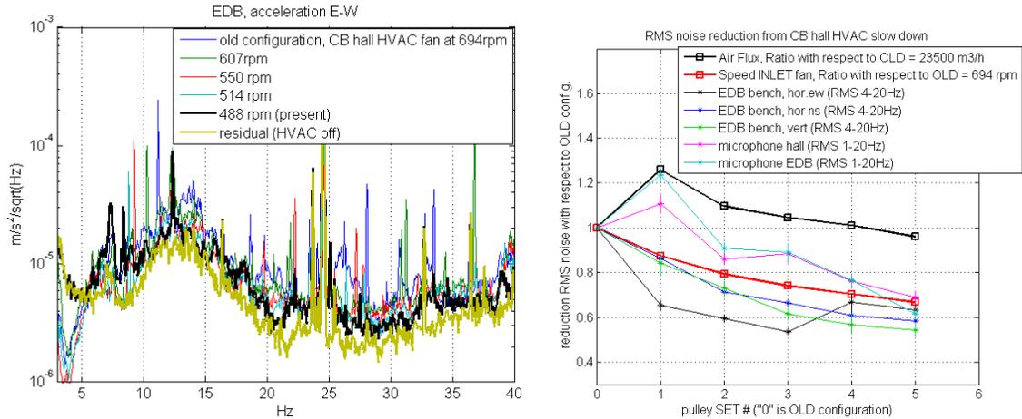
**Figure 3.** Measured reduction of a seismic noise (LEFT) on EDB consequent to the slow down of fans of the Central hall air conditioning. Residual noise is the difference of black and yellow curves. (RIGHT) RMS noise reduction of seismic and acoustic noise in CB hall and Detection, as function of the air flux and speed of HVAC inlet fan.
