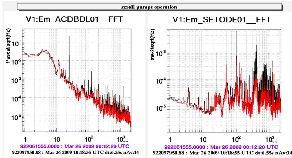
**Figure 10.** Acoustic and seismic noise produced by the vacuum scroll pump serving the DET tower. Black curves are with pump on, red curves with pump off. Left plot is a microphone on the EDB, right plot is a seismometer on the DET tower output window.
