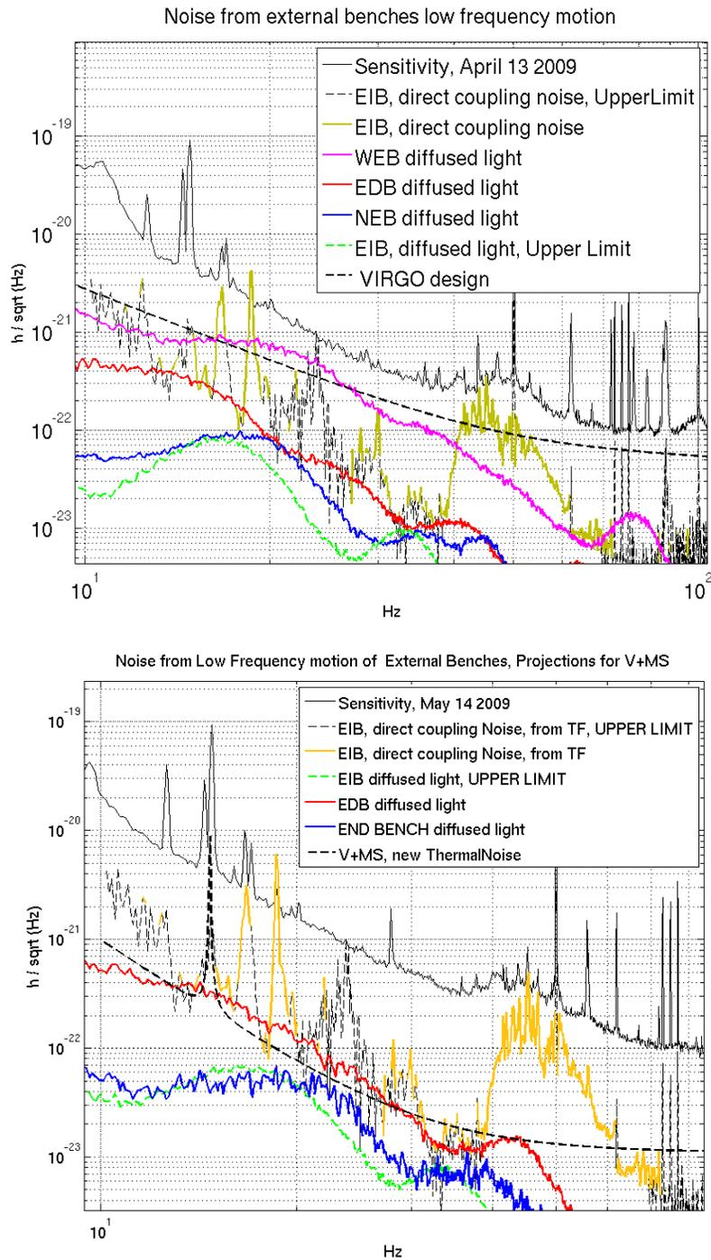
**Figure 5.** (TOP) Projection of environmental noise coupling through motion of external benches, as of April 2009. (RIGHT) Tentative projection of the same noises for V+MS.
