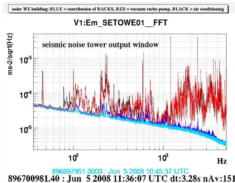
**Figure 11.** Seismic noise produced by the WE vacuum turbo-molecular pump measured at the tower output flange (red to blue). No bellow is installed on this pump. Also shown is the noise contribution from the air conditioning (black to red), and part of the contribution of the racks (blue to cyan). The cyan curve is essentially measuring sensor noise.
