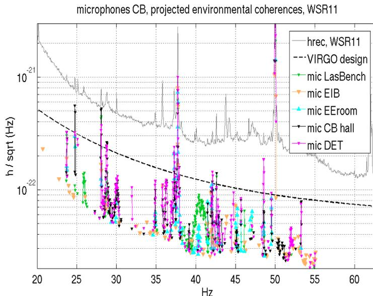
**Figure 9.** Projected coherence between dark fringe and microphones in the Central Building during WSR11 run (Feb. 2009). Measured coherences are multiplied by hrec and plotted. Some peaks have been identified associated to vacuum racks close to INJ. We suspect most of these peaks to be due to racks.
