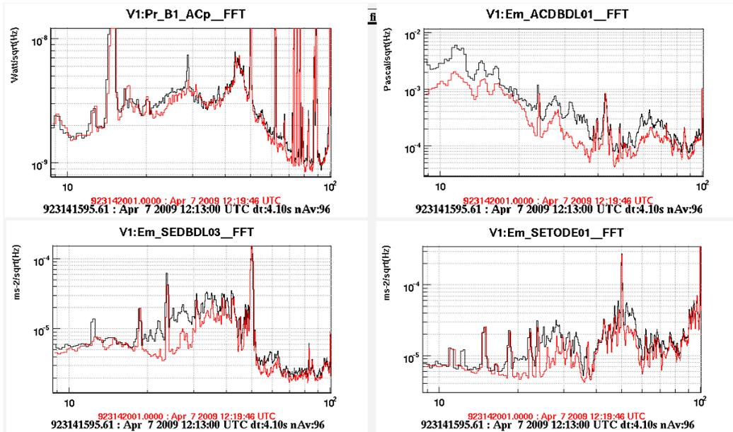
**Figure 4.** Effect of switching off the CB hall HVAC machine (April 2009): black curves correspond to the machine ON, red curves are with machine OFF. Upper left plot is the dark fringe, Upper right is the microphone on EDB, Bottom left is one seismometer on EDB and Bottom right is one seismometer on DET tower output window.
