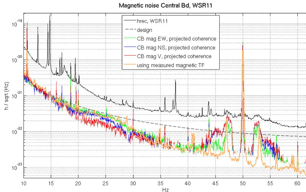
**Figure 13.** Projection of magnetic environmental noise coupling to mirror magnets in the central experimental hall. WSR11 data. The noise around 50Hz is due to the switching heating resistance of the MC building HVAC, as explained in Sec. 4.1 item (4).
